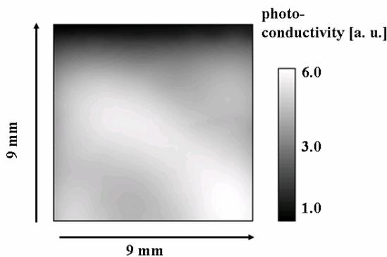
**Fig. 3** MDP mapping ( $9 \times 9 \text{ mm}^2$ ) of the as-grown Fe-doped SI-InP sample B (excitation energy: 1.9 eV, penetration depth of light: approx. 200 nm). It indicates the distribution of defects with a noticeable influence on the electrical characteristics of the wafer at room temperature.
