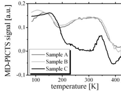
**Fig. 1** Comparison of MD-PICTS spectra of as-grown Fe-doped SI-InP samples from different crystal positions (excitation energy: 1.3 eV, penetration depth of light: approx. 600 nm). The samples differ in their characteristic defect levels.
