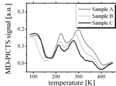
**Fig. 2** Comparison of MD-PICTS spectra of wafer annealed Fe-doped SI-InP samples taken from the same wafers as the as-grown samples (excitation energy: 1.3 eV, penetration depth of light: approx. 600 nm). All spectra show an equivalent set of defect levels.
