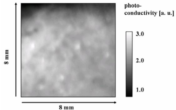
**Fig. 4** MDP mapping ( $8 \times 8 \text{ mm}^2$ ) of the wafer annealed Fe-doped SI-InP sample B (excitation energy: 1.9 eV, penetration depth of light: approx. 200 nm). The granular structure of the electrical inhomogeneities is possibly due to the distribution of a few prominent defect levels.
