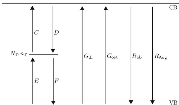
**Fig. 1** Semiconductor model with one artificial defect level and all considered band-band and defect-band interactions
