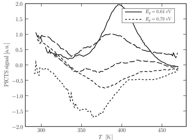
**Fig. 2** Measured positive and negative EL2 PICTS-peaks. Peaks from the experimental data [14] have been re-calculated for convenience (here using an initial delay  $t_1 = 30 \mu s$  in PICTS spectra generation)
