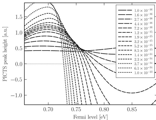
**Fig. 5** Dependence of the peak height (positive or negative) on the Fermi level and the RC cross sections  $\sigma_{n,p}$ (RC) (values in the legend in  $\text{cm}^2$ ). Peaks are calculated for  $t_1 = 30 \mu\text{s}$  from the same simulation data as in Fig. 4
