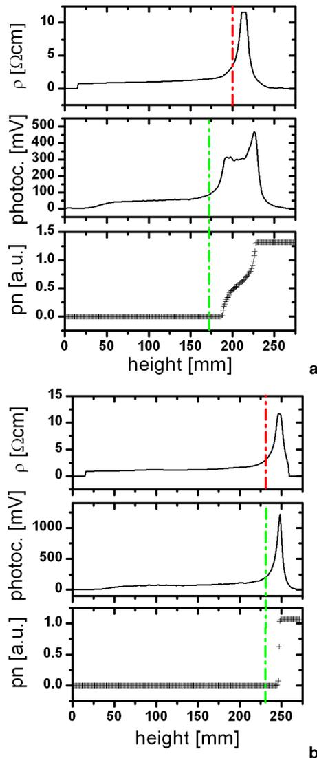
**Figure 6** Average photoconductivity linescan of the bricks shown in figure 4 along with the corresponding output of the pn detection algorithm and the resistivity linescan measured in the middle of the brick
