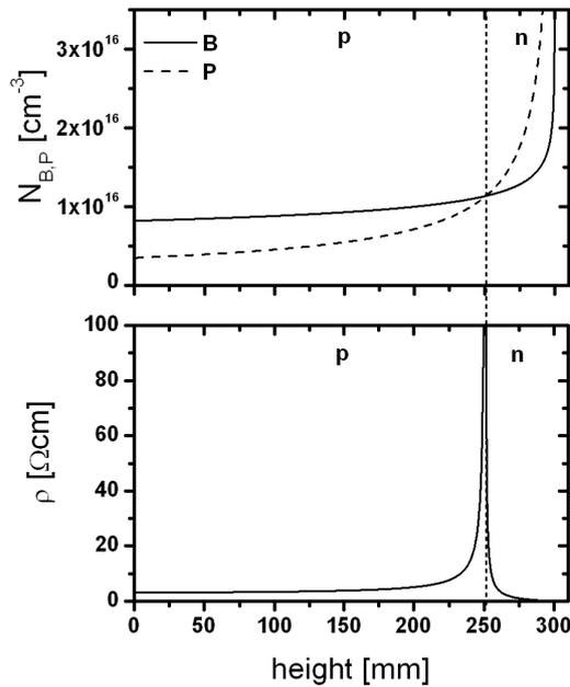
**Figure 1 Typical concentrations of boron and phosphorus versus the brick and the resulting resistivity versus brick height determined by the Scheil equation with  $C_{0,B} = 10^{16} \text{ cm}^{-3}$ ,  $k_B = 0.82$  and  $C_{0,P} = 10^{16} \text{ cm}^{-3}$ ,  $k_P = 0.35$**
