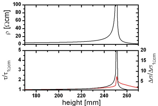
**Figure 3 simulated resistivity linescan for a pn junction and resulting changes in the measured lifetime (red) and photoconductivity (black) compared to the values at  $1 \text{ Ohm}\cdot\text{cm}$**
