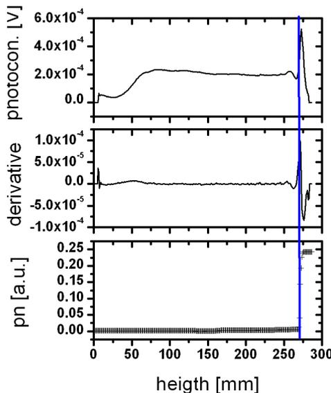
Figure 4 Exemplary photoconductivity linescan, its derivative and the resulting output of the detection algorithm
