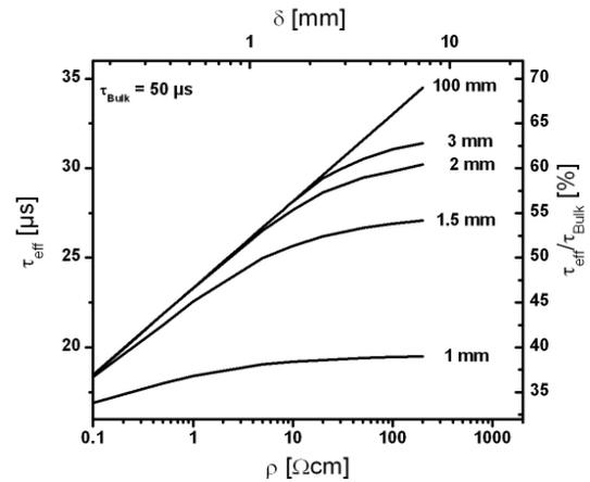
**Figure 2 Effective lifetime and relative deviation from bulk lifetime versus resistivity and skin depth for different sample thickness**
