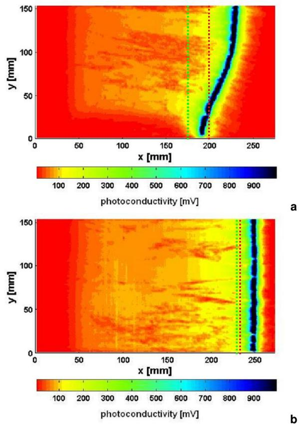
Figure 5 Exemplary photoconductivity maps of two mc-Si bricks with indicated detection height of the algorithm (green line) and height at which the resistivity linescan rises above  $3 \Omega\text{cm}$  (red line)
