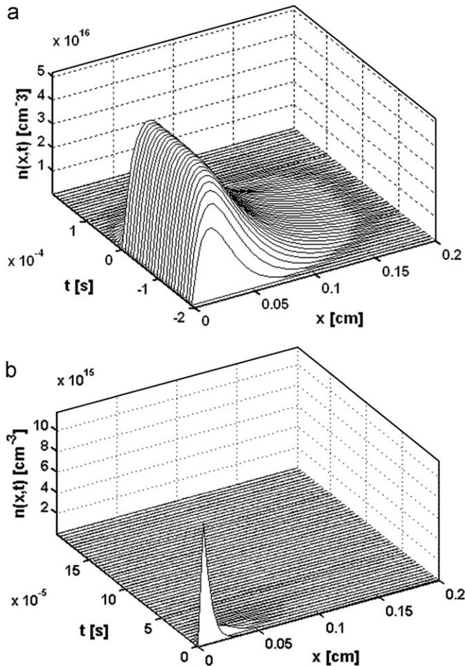
**Fig. 2.** Carrier profile in a 2 mm thick sample with  $N_{\text{dot}}=10^{16} \text{ cm}^{-3}$  at 300 K for a typical MDP (a) defined by light pulse duration of 200  $\mu\text{s}$ ,  $\lambda=978 \text{ nm}$ , microwave frequency  $\nu=9.4 \text{ GHz}$  and a  $\mu\text{PCD}$  (b) measurement defined by light pulse duration of 200 ns,  $\lambda=904 \text{ nm}$ ,  $\nu=10.4 \text{ GHz}$ , for both cases FeB was used as the recombination center as defined in [9].
