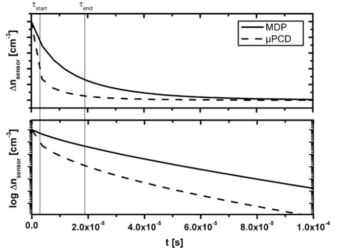
**Fig. 4.** Normalized transient of sensor-weighted carrier density for MDP and  $\mu\text{PCD}$  conditions.
