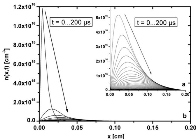
**Fig. 3.** Time dependent behavior of the carrier profiles of MDP (a) and  $\mu\text{PCD}$  (b) measurement with  $N_{\text{dot}}=10^{16} \text{ cm}^{-3}$ .
