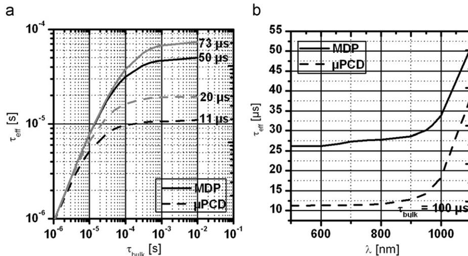
**Fig. 5.** Evaluated effective lifetimes as a function of bulk lifetime (a) for both methods and  $N_{\text{dot}} = 10^{16} \text{ cm}^{-3}$  (black) and  $N_{\text{dot}} = 10^{15} \text{ cm}^{-3}$  (gray); evaluated effective lifetimes as a function of the exciting laser wavelength (b).
