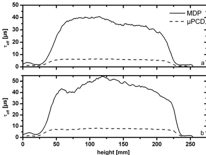
**Fig. 6.** Exemplary measurement results for two mc-Si ingots with  $\rho = 1.31 \Omega\text{cm}$  (a) and  $\rho = 0.92 \Omega\text{cm}$  (b).
