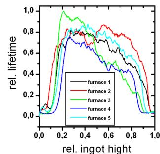
**Figure 4:** lifetime average versus ingot height for 5 ingots grown in different furnaces
