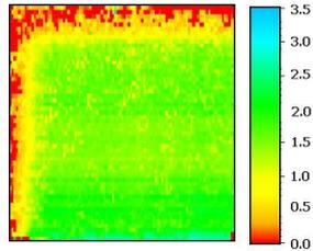
**Figure 1:** lifetime map of a mc-Si wafer from the edge of a cast ingot
