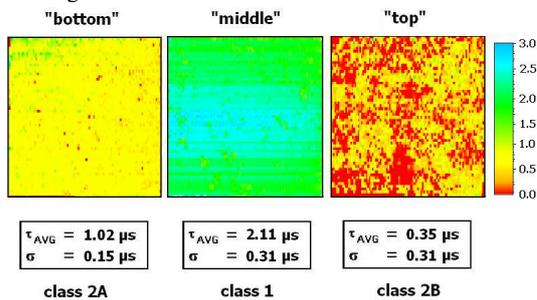
**Figure 2:** Exemplary classification of three wafers of bottom (a), the middle (b) and top(c) of an ingot.
