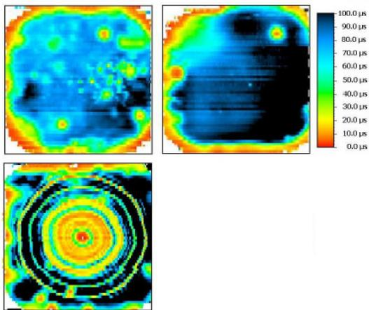
**Figure 6:** examples of an inhomogeneous passivation and striations
