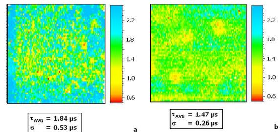
**Figure 3:**  $\text{Si}_3\text{N}_4$  and SiC segregates (a); microcrystalline wafer (b)
