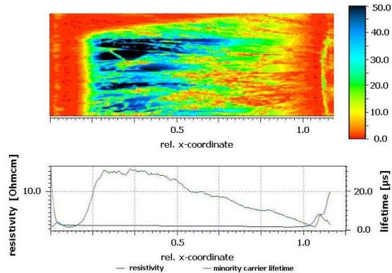
**Figure 7:** exemplary lifetime map of an ingot with a change in conduction type
