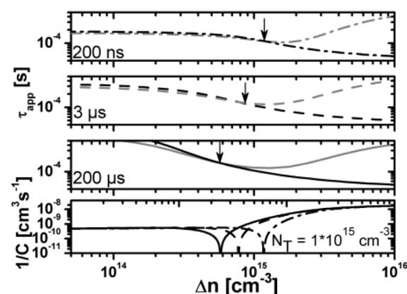
**Fig. 4:** Simulated apparent lifetime curves for FeB (black) and Fe<sub>i</sub> (grey) for three different laser pulse lengths; resulting reciprocal calibration factor versus injection
