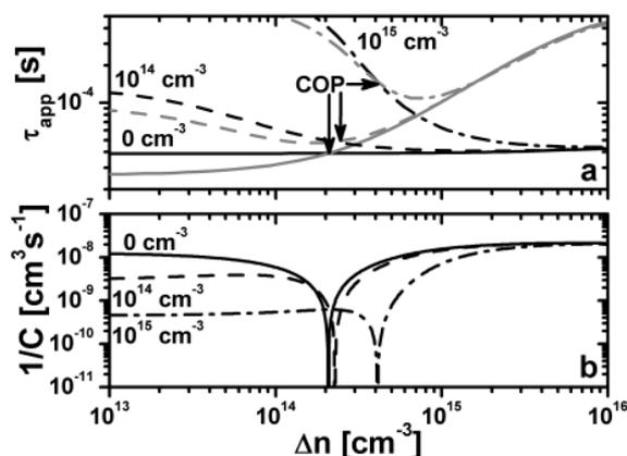
**Fig. 3:** Simulated apparent lifetime curves for FeB (black) and Fe<sub>i</sub> (grey) for three different trap densities (a); resulting reciprocal calibration factor versus injection (b)
