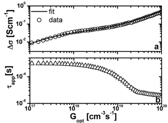
**Fig. 2:** Measured photoconductivity and fit curve versus  $G_{opt}$  (a); apparent lifetime versus  $G_{opt}$  (b); determined trap parameter:  $N_T = 8 \cdot 10^{14} \text{ cm}^{-3}$ ,  $E_A = 0.387 \text{ eV}$
