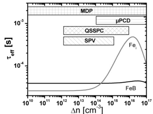
**Fig. 1:** Injection dependent lifetime curves for FeB and  $Fe_i$  and injection ranges measurable by MDP,  $\mu$ PCD, QSSPC and SPV
