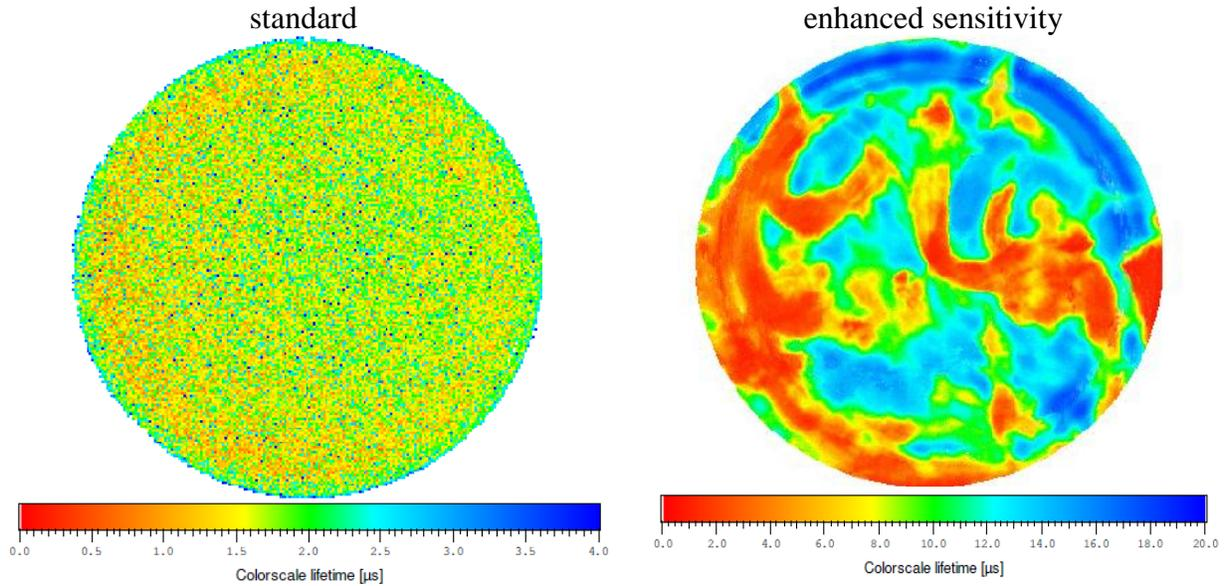
**FIGURE 2.** Example of enhanced sensitivity by a factor of 100; 50  $\mu\text{m}$  p-doped silicon epilayer on highly doped silicon substrate, passivated with thermal oxide
