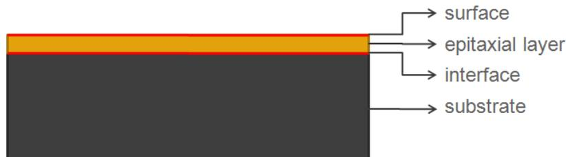
**FIGURE 1.** Scheme of the recombination sites of a sample with an epitaxial layer
