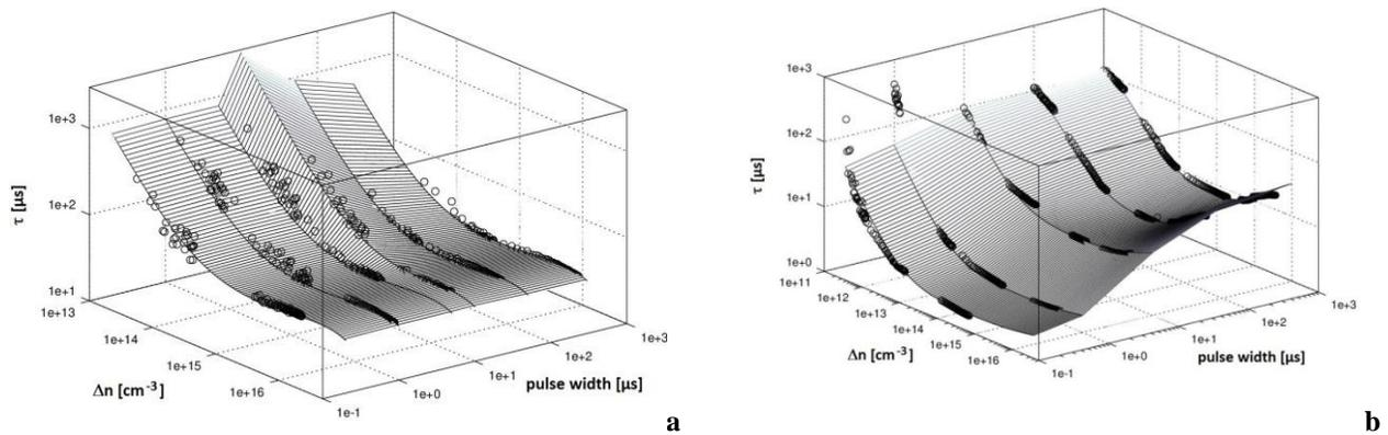
**FIGURE 3.** Injection dependent lifetime curves with different pulse widths of a 6  $\mu\text{m}$  n-Si epitaxial layer passivated by a thermal oxide (a) and of a 30  $\mu\text{m}$  n-Si epitaxial layer passivated by amorphous Si (b). The drawn lines are just to guide the eye.
