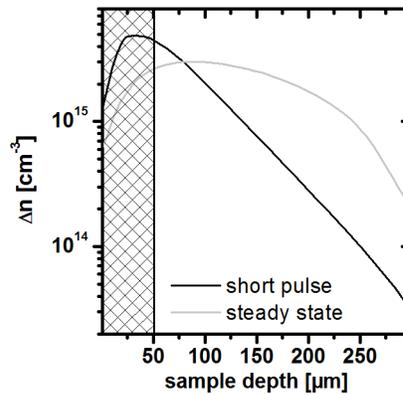
**FIGURE 1.** Simulated carrier profiles in a 300  $\mu\text{m}$  thick sample that developed after a short pulse (200 ns) excitation and a steady state (200  $\mu\text{s}$ ) excitation; the carrier profile right after switching off the light is shown
